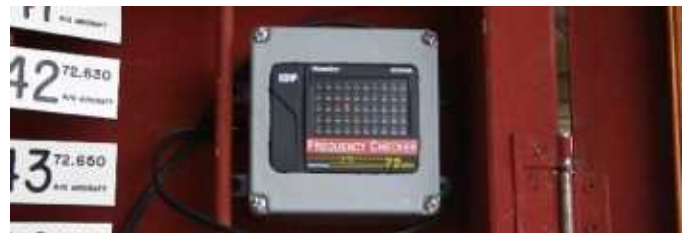
woodworking power-tools; on-site frequency-checker to scan all 72MHz aircraft channels for interference.
